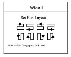
Note: Cabinet routing mode: Series mode between receiving cards should ensure that the direction of the two cable is the same.
