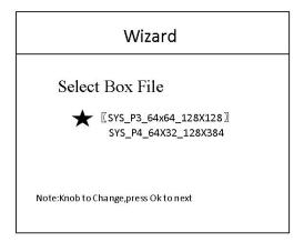
Note: The box files need to be imported into the equipment through the upper computer software.
